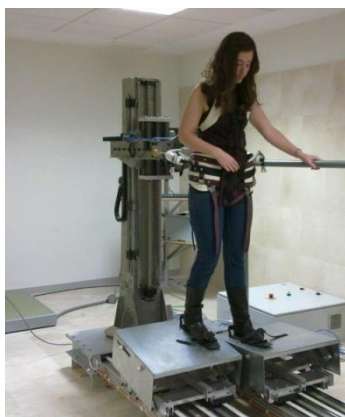
Prototype of a robot for the rehabilitation of walking in patients with brain damages ( http://www.walkx.com/ )
