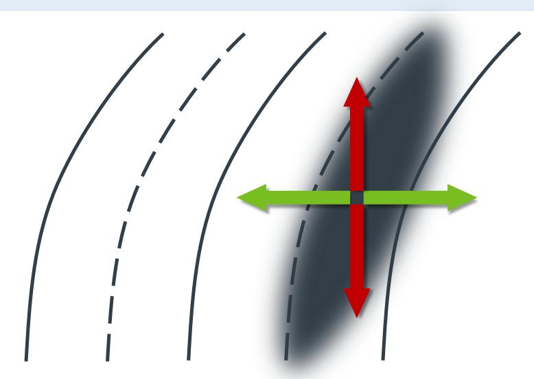
High confidence in lateral direction: Position can safely be mapped to the correct lane even with high uncertainty in driving direction.
