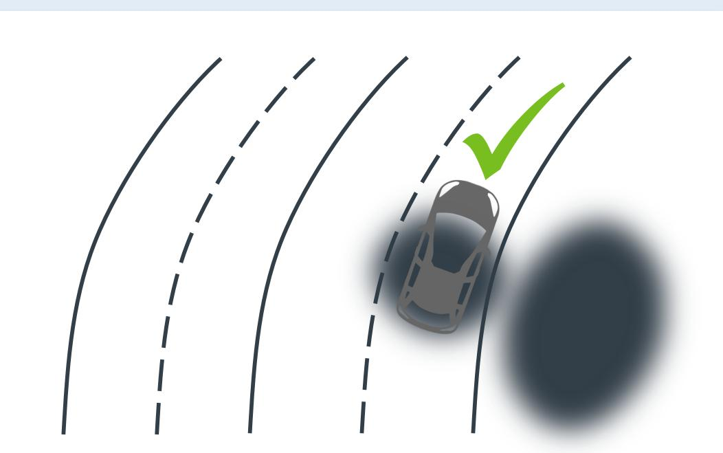
NAVENTIK: Signal reflections are statistically tracked in the receiver. The true vehicle position is covered by the multimodal error envelope.
