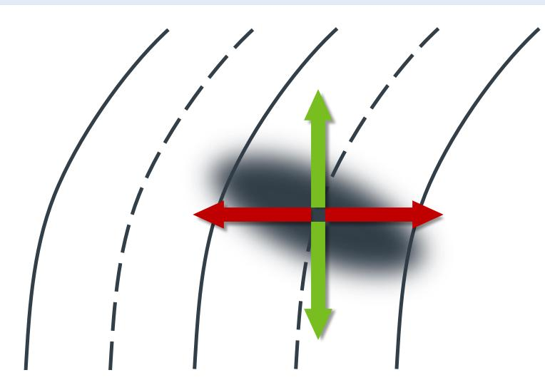
High confidence in driving direction: Driving instructions can be precise in terms of distance to the next event but should not provide lane level recommendations.
