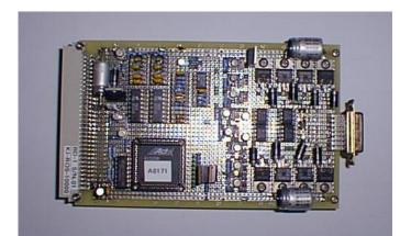
ROSETTA (OG) Breadboard of drill and carousel control for Shark subsystem
