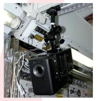
ELITE-S2 camera in the USLab of ISS
