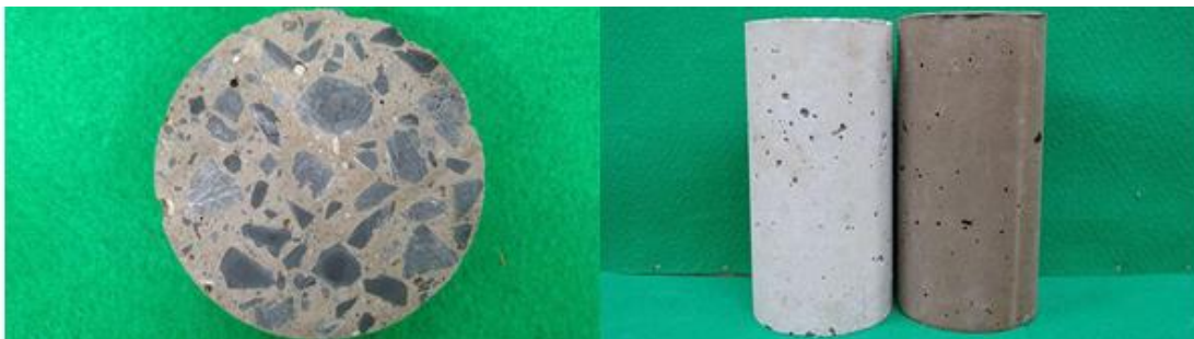
(Left) Lignin cleat cross section / (Right) Comparison with ordinary concrete Image from Obayashi Corporation website
