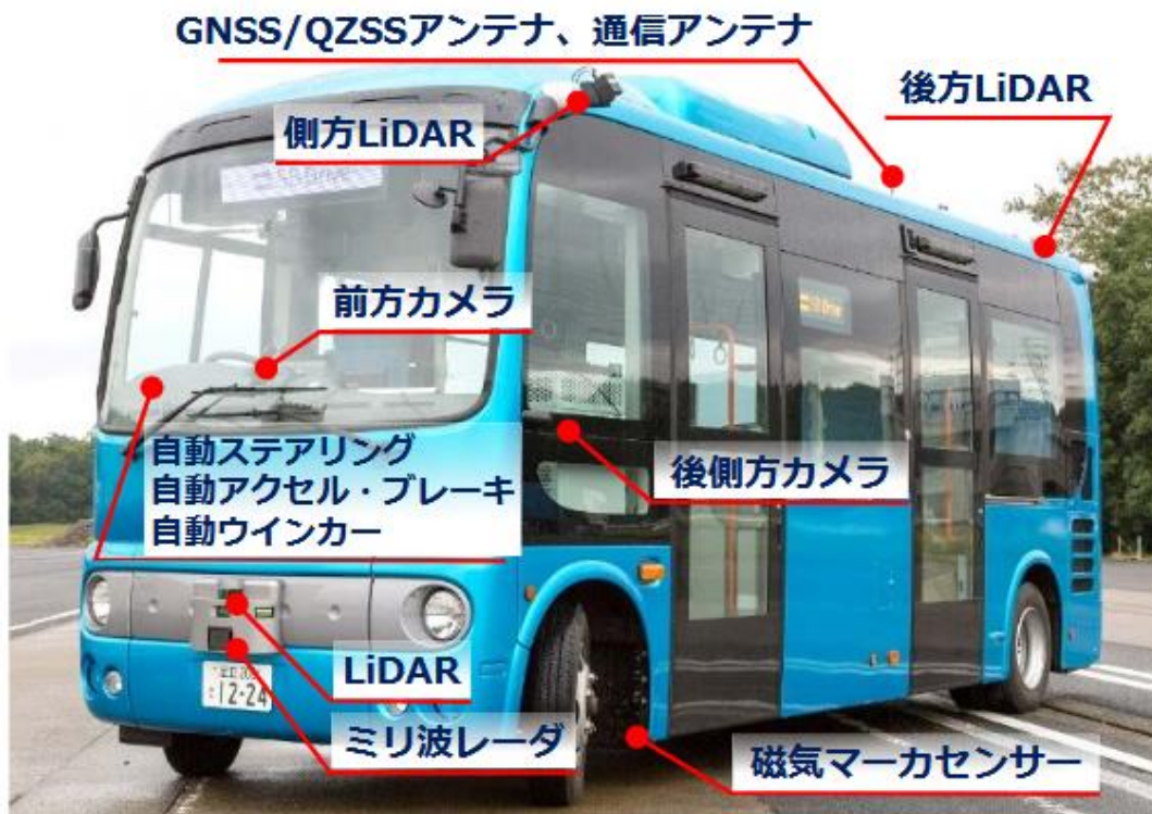
Experimental vehicle to be used in demonstration test
