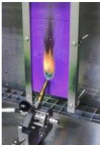
Example of ignition-property tests for photo voltaic cell modules Photos provided by the Japan Electrical Manufacturers' Association
