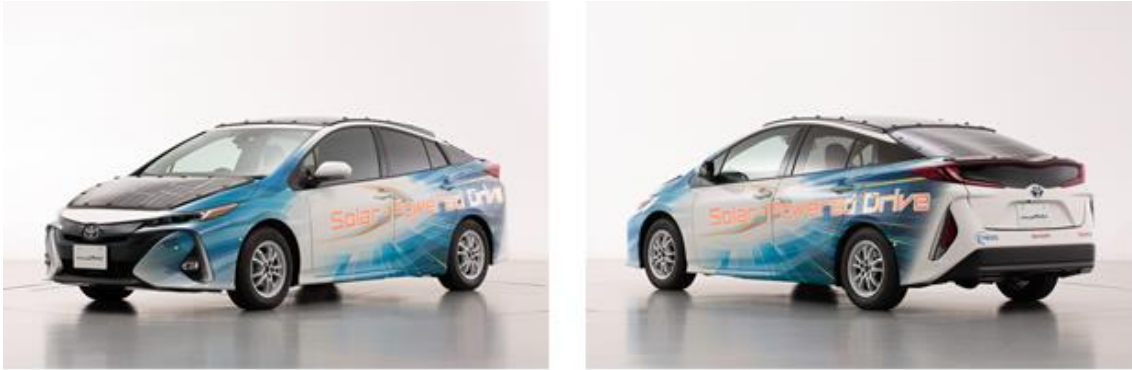
Prius PHV Test Car with Solar Cell Panels
