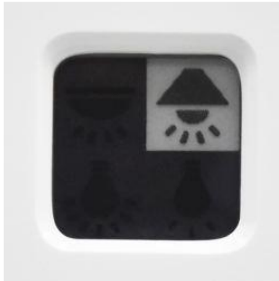
Newly developed electronic paper display. Segmented EPD technology enables ultralow power consumption.
