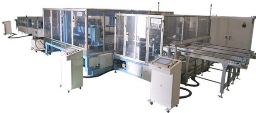
From NPC website: Automatic solar panel dismantling device / line
